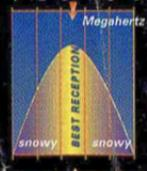
When TV signals are tuned at the TV channel's center frequency, optimum tuning has been achieved.
